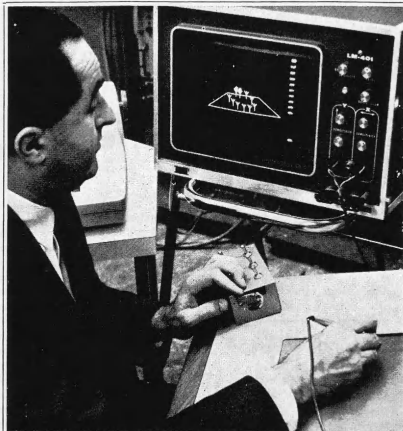
The display on the screen and the electronic pencil held by the demonstrator are controlled by a digital computer (large metal cabinet containing electronic equipment is seen in part at left). The demonstrator indicates the patterns he wants by writing numerals on an electronically sensitive plate. The computer translates the information to the screen immediately in the form of stick figures. These, says Mr. Noll, can eventually be anatomically more detailed.
